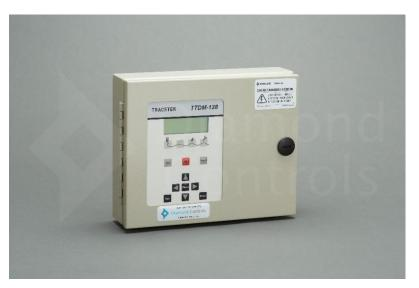
When liquid is detected on any of the sensors, the TTDM-128 sounds an alarm, closes relay contacts, turns on a front panel LED and displays the circuit identification and location of the leak on the alphanumeric display. The leak detection event is logged to a non-volatile event history file. All status and event information is made available via the front panel keyboard or RS232/RS485 modbus digital communication to a host computer, PLC or plant/building automation system.
