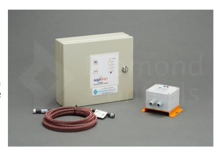
The panel display includes LED's for each of the four zones. In the event of a leak the alarm sounds, and the LED indicates the zone where the leak has occurred. The operator silences the alarm by pressing the mute button. A red flashing leak LED indicates the leak has cleared and requires the reset button to be pressed. In the event of multiple alarms, the panel will not reset until all the leaks have been cleared. Pushing reset will also reset the volt free contacts.
